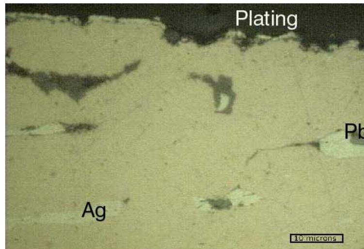
**Figure 1:** A characteristic example of the metallographic structure of the coins (coin BM259).
