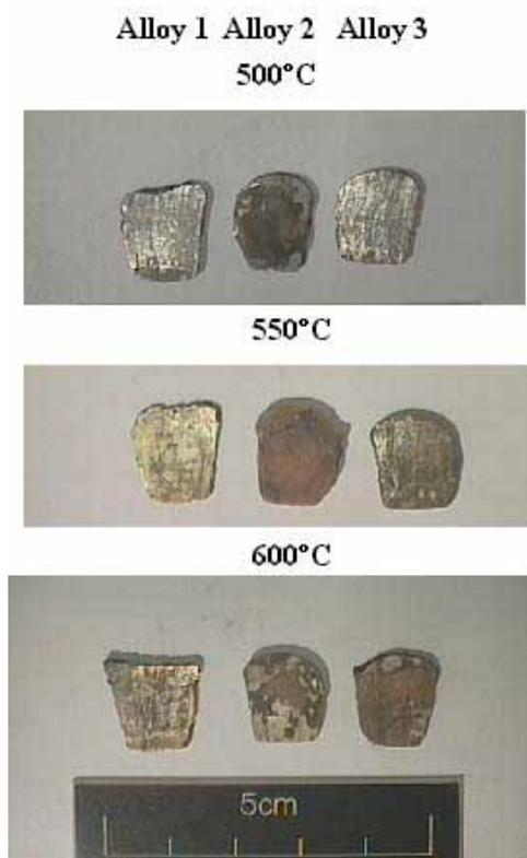
**Figure 4:** The coupons after heating for 20 min in 500°C, 550°C and 600°C.
